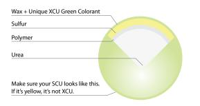
The coating is what makes XCU better. Because the coating on XCU is more consistent and has improved durability, the granules maintain integrity during transportation, blending, bagging and application. That's important, since broken granules release too much nitrogen up front, which risks environmental loss, surge growth and shorter residual feeding.
